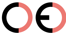
False CE Mark (too far)
